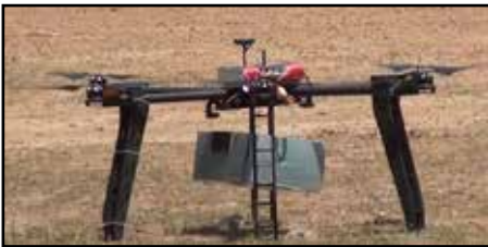
Fig : Autonomous package delivery drone of the University of Moratuwa delivering a package of 1kg
