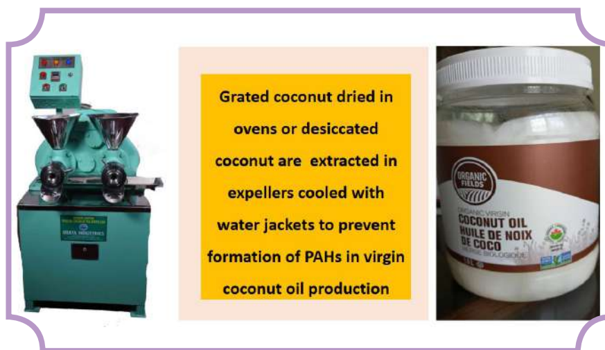
Figure 3: Water jacketed oil expellers used for virgin coconut oil to prevent formation of PAHs
