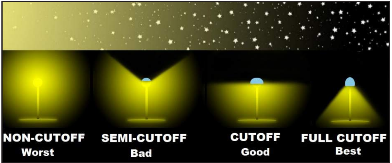
Figure 03 : Cutoff Classification of Light Fittings
