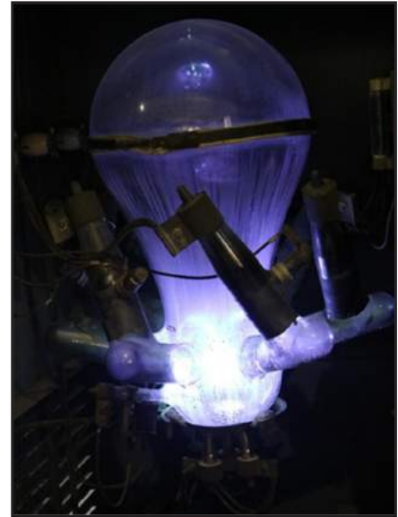
Figure 03 : Probably the last operating mercury arc rectifier in the world; this is still serving students at the Department of Electrical and Electronic Engineering, University of Peradeniya
